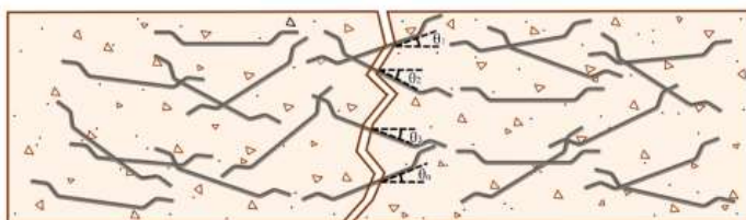
Fig 5. Schematic illustration of fiber alignment evaluation in concrete [85].
