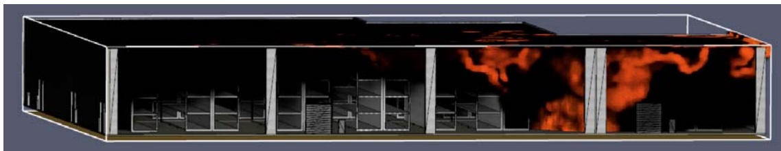
Fig. 9. Vertical smoke stratification after 600 seconds
