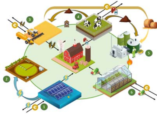
Figure 2. Proposed farm concept. 1-floating photovoltaic panels installed on the irrigation lake, 2-fixed point irrigation system, 3-crop harvesting, 4-livestock farming, 5-biogas plant, 6-greenhouse horticulture
