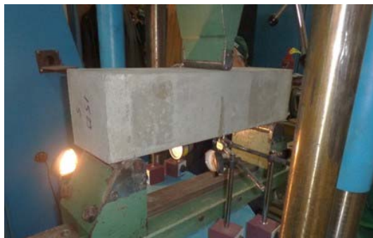
Fig. 9 Experimental device used for 3-point bending test
