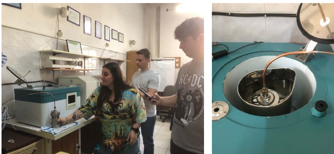
Fig 7. Preparation of the commissioning of the calorimetric bomb
