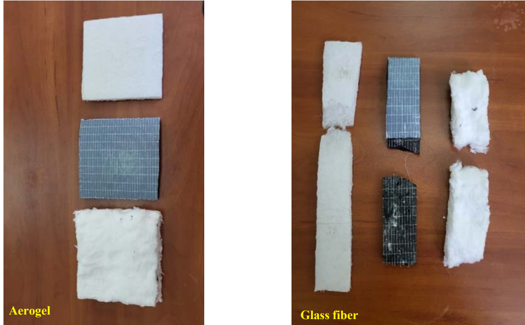
Fig. 4. Tested materials before and after tensile strength testing
