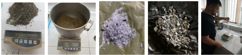
a) cement, b) sand, c) PV crushed, d) pieces of PV, e) water
