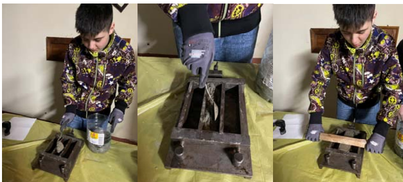
Figure 5. Pouring and compacting the mixture
