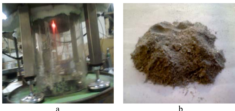
Fig. 1. Details on the atomization of molten aluminum a – the atomization area of the plant; b – batch of aluminum granules (Reproduced by permission of Junkoeko SRL Slobozia, Romania).
