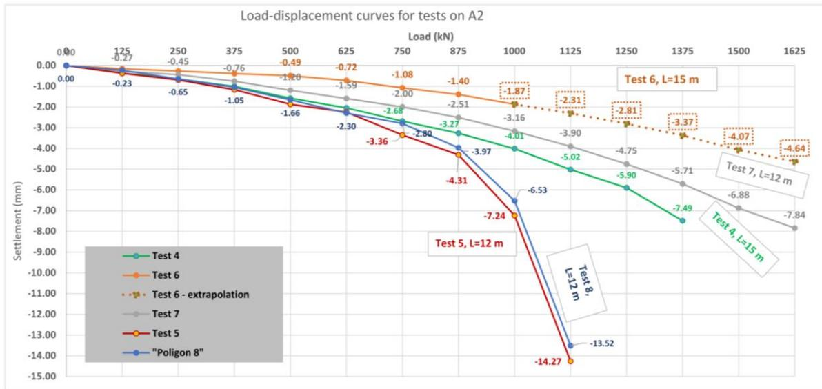
Figure 4. Load-settlement curves for all tests (5 piles).
