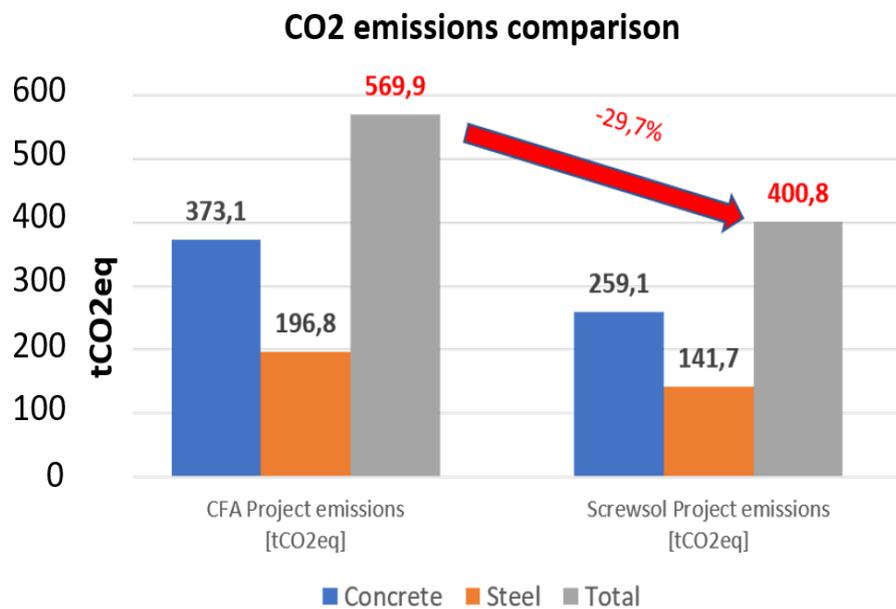
Figure 7. CO2 emissions for CFA and Screwsol.
