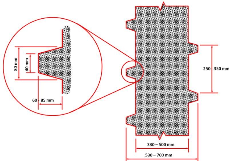
Figure 1. Screwsol pile longitudinal section and thread details.
