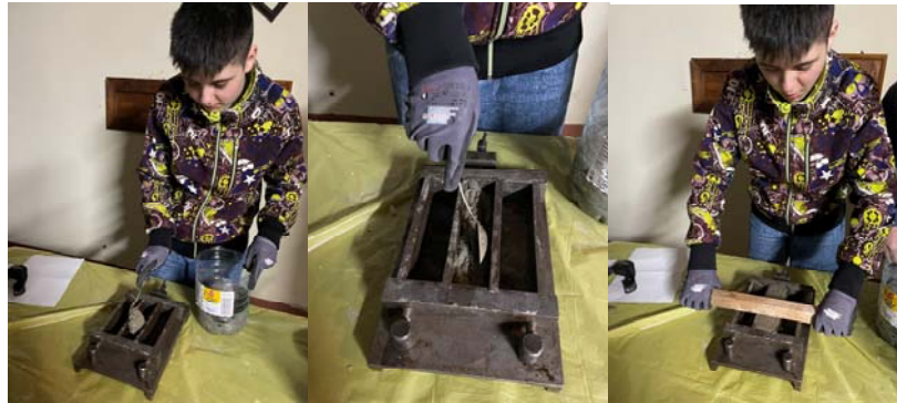
Figure 5. Pouring and compacting the mixture
