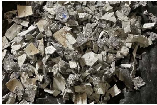
Figura 3. Material obtained after manual cutting of PV-pieces (glass + plastic)
