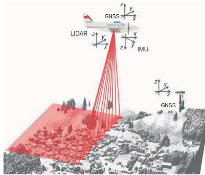
Fig. 1. Principle of airborne laser scanning [26]
