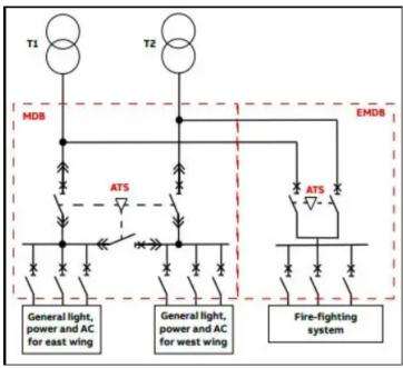
Fig. 2. ATS backing up supply for loads [4] T1, T2 – Divided supply routes, MDB – Main Distribution Board, EMDB – Emergency Main Distribution Board
