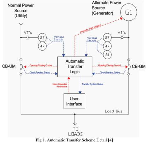
CB-UM/GM – Circuit Breaker Utility/Generator Module, VT's – Voltage Transformers, 27 – Undervoltage indicator, 47 – Negative sequence voltage, 81 – Frequency indicator
