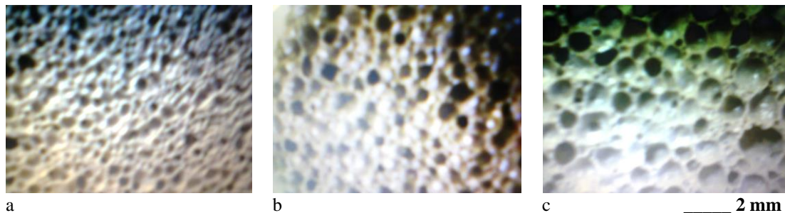
Fig. 3. Microstructural configuration of the cellular glass samples a – variant 1; b – variant 2; c – variant 3.
